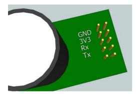
The Rx and Tx pins are normally high, suitable for direct connection to a UART. If the sensor is to be read by a true RS232 device (such as a PC), it is necessary to pass through a level converter to step up/down the voltage and invert the signal.
