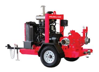
Global Pump<sup>®</sup> High Performance Trash pumps are specifically designed to effectively handle a wide-range of liquids from water to sewage and sludge that can contain solids and other material.
